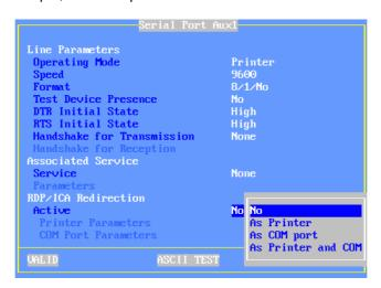
Set the 'Active' parameter to 'As COM port' or 'As Printer and COM'. Then select 'COM Port Parameters' and press <Space>. The following box is displayed:
