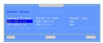
**Example 2**: router 1 is used to reach both networks (192.168.2.xxx and 192.1.1.xxx):
