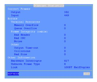
**Correct Frames**: "Output" and "Input" are the number of correct frames (transmitted and received)
