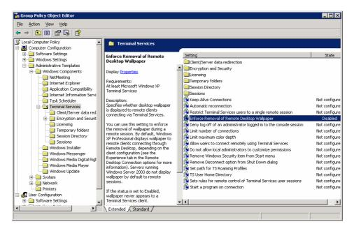
Expand the tree to [Computer Configuration]-[Administrative Templates]-[Windows Components]-[Terminal Services]. Set the parameter "Enforce Removal of Remote Desktop Wallpaper" to "Disabled".
