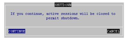
If the user confirms, all active connections (screens and auxiliary ports) are closed. A few seconds later, the user is informed that the AX3000 may be turned off.
