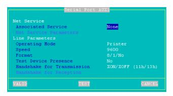
The **[TEST]** button allows communication between the AX3000 auxiliary port and the device to be tested. Whatever the auxiliary port status (TCP/IP connection established or not), when this button is 'pressed', data is sent from
