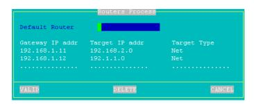
**Example 2**: router 1 is used to reach both networks (192.168.2.xxx and 192.1.1.xxx):
