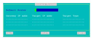
**Default Router**: to specify a default router enter its IP address. If a default router is not required, leave this field blank. If 'Default Router' is enabled in the AX3000 Interface box, this parameter is automatically supplied by DHCP and cannot be accessed.
