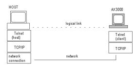
On the host a network 'package' is used to manage the Ethernet controller with Telnet (host) and TCP/IP protocols. Each connected terminal is addressed via a pseudo-terminal (ptty).
