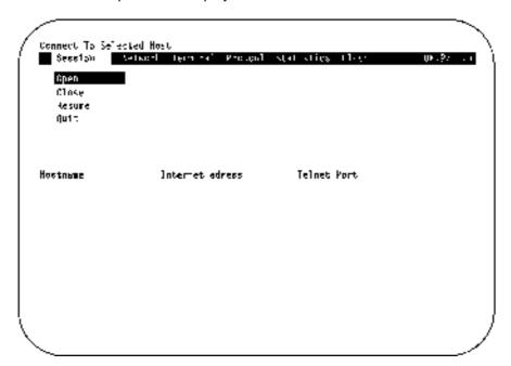
The TCP/IP Set-Up appears as a menu bar and several pull-down menus. Within these menus, use the arrow keys to select a function and confirm it by pressing the **<RETURN>** key.
