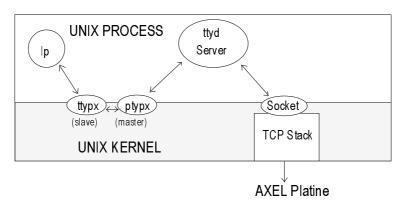
In this example, the UNIX device being used is a pseudo-terminal. This bidirectional device allows connection of a PostScript printer (or a serial terminal).
