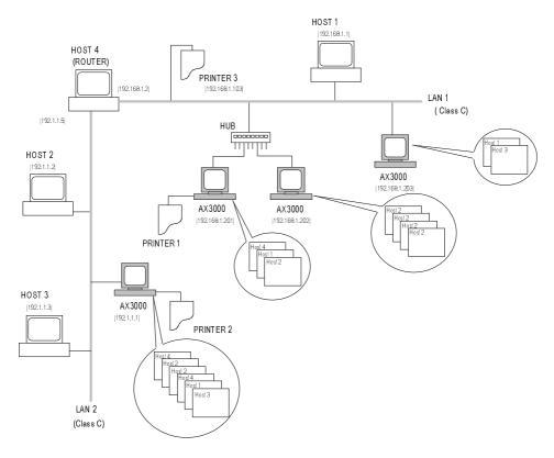
In this example, two distinct local area networks are linked. Host 1 is attached to network 1 (class C) while hosts 2 and 3 are attached to network 2 (class C). Host 4 is attached to networks 1 and 2 and acts as a router between them.
