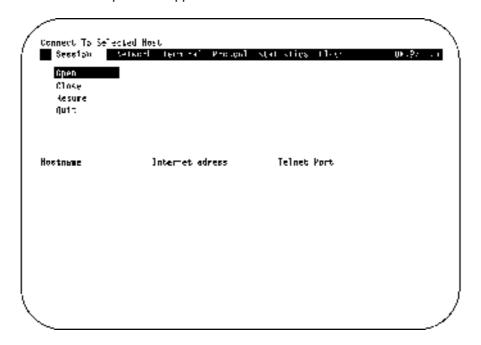
Move through the menu with arrow keys. Information, relating to each command selected, will be automatically displayed at the bottom of the screen.
