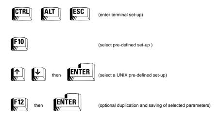
The pre-defined set-up (**<F10>** option) automatically initiates main terminal parameters for the corresponding session. If necessary, each individual terminal parameter (number of lines, columns, function keys, etc) can be modified individually.
