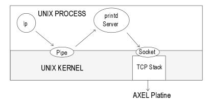
In this example, the UNIX device being used is a named pipe (uni-directional device), but a pseudo-terminal could be used also.
